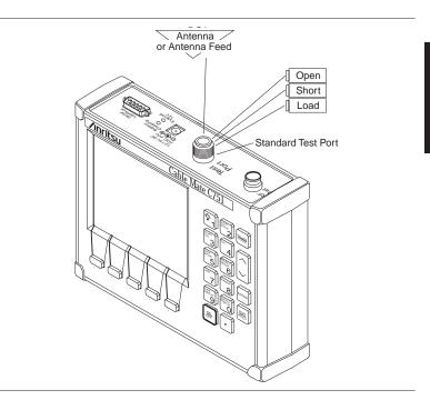
Figure 2-9. Measurement/Calibration Test Setup
