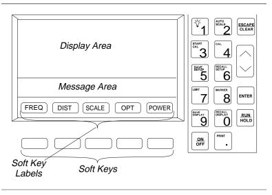
Figure 2-2. Cable Mate Front Panel Display Layout
