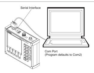
Figure 3-3. Equipment Setup for Cable Mate Tools Operation
