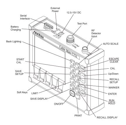
Figure 2-1. Cable Mate Controls and Connectors
