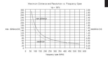
Figure 2-10. Maximum Distance and Resolution vs Frequency Span
