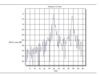
Figure 2-4. Rectangular Windowing Example
