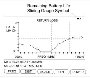
Figure 2-8. Battery Monitor
